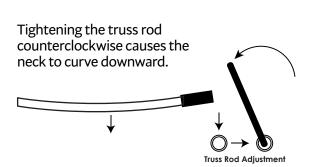
Tightening the truss rod clockwise causes the neck to curve upward.
