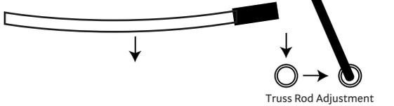
Tightening the truss rod clockwise causes the neck to curve upward.
